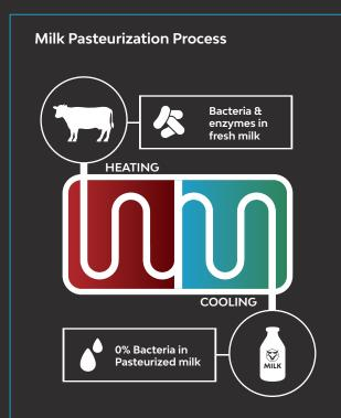
Pasteurization is the process of heating milk up and then quickly cooling it down to eliminate certain bacteria and enzymes. Milk treated with pasteurization or HTST is labeled as pasteurized while milk treated with UHT is labeled as "ultra-pasteurized.
