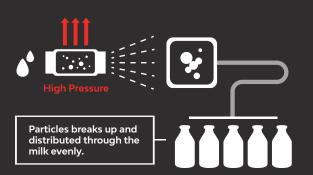
Homogenization is the process during which milk is squirted through a special machine under very high pressure. This breaks up fat particles and makes them small enough to disperse through the milk evenly.
